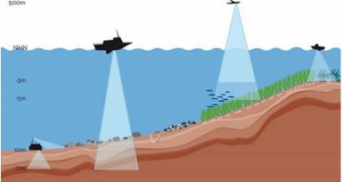
Overview of the acoustic and laser remote sensors and habitats to be investigated in ECOMAP. Carrier platforms are ship vessels, in situ monitoring devices on the seabed, and aircrafts.
